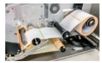
Unique light barrier bar for automatic recognition of different label sizes and label geometries.
